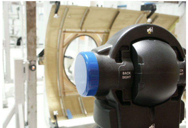
Utilizing Laser Tracker Services during fuselage construction.
