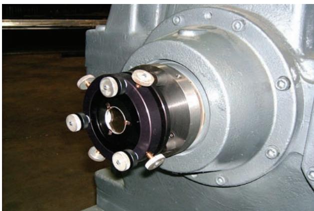
OASIS Alignment Set-Up - Magnetic Spindle Mirror for establishing reference at back end of Reducer Output
