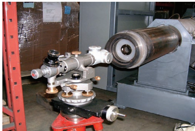
OASIS Optical Instrument Set-Up with Die End target in barrel mouth. Instrument is bucked-in to Spindle Mirror.
