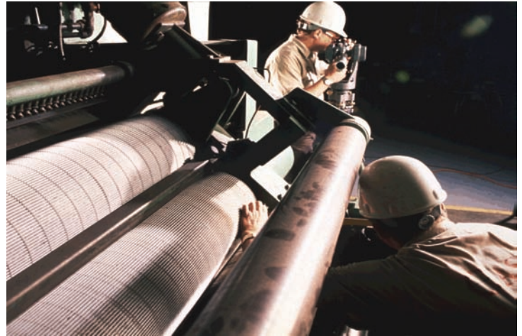
OASIS engineers recording perpendicular readings on a single facer roll.
